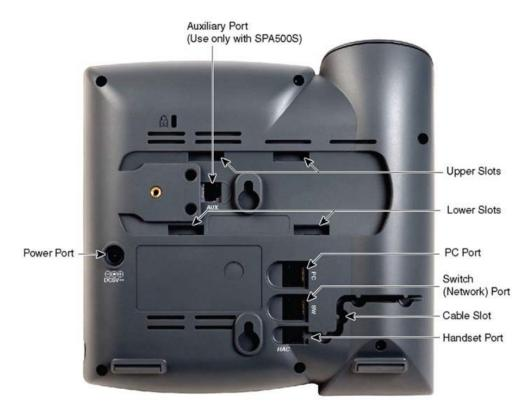
Step 1. Turn the phone body over to expose the ports on the back of the unit.
