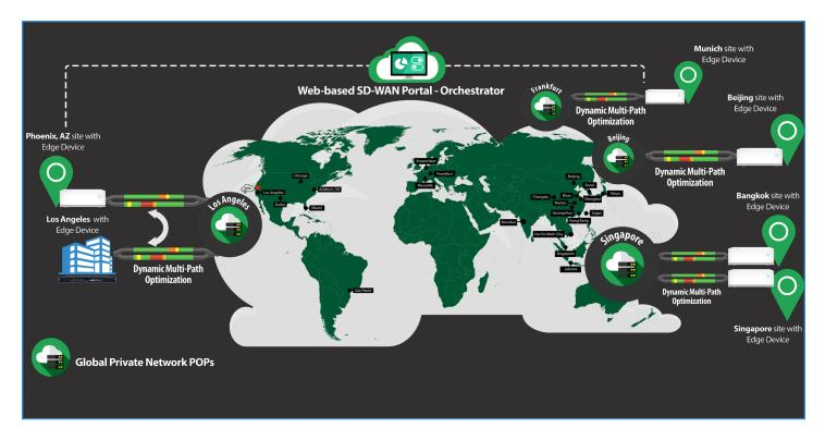
AireSpring PoPs are fully-meshed to provide a failsafe and highly resilient network that ensures reliable and consistent global connectivity. The PoPs directly connect branch offices and data centers, to cloud applications, compute resources, and virtualized services.
